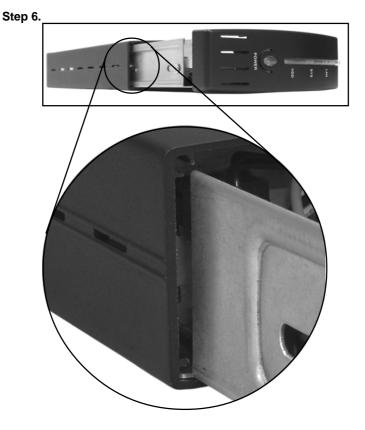
(1) Position the back of the Inner Cradle Assembly into the head of the Body Outer Cover.
